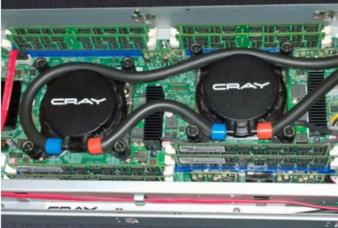
Figure 8- A look at server for a Cray CS400 supercomputing cluster, which is cooled with an Asetek system that brings warm water to the chip. (Photo: Rich Miller)
