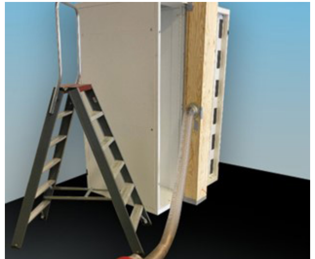
Testing setup to quantify air leakage for the brushes
