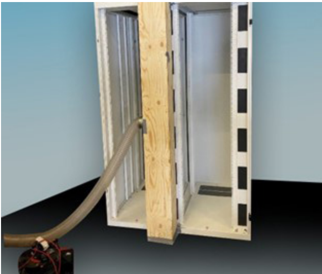
Testing setup to quantify air leakage for the brushes
