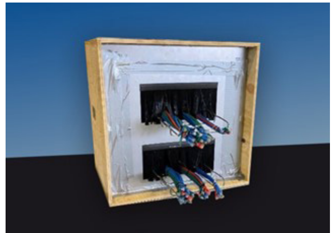
Testing setup to quantify air leakage for the brushing
