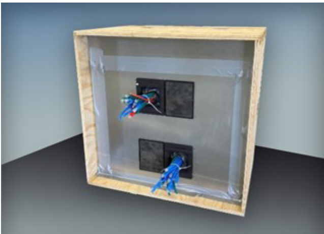
Testing setup to quantify air leakage for the Cable Entry Seal accessory
