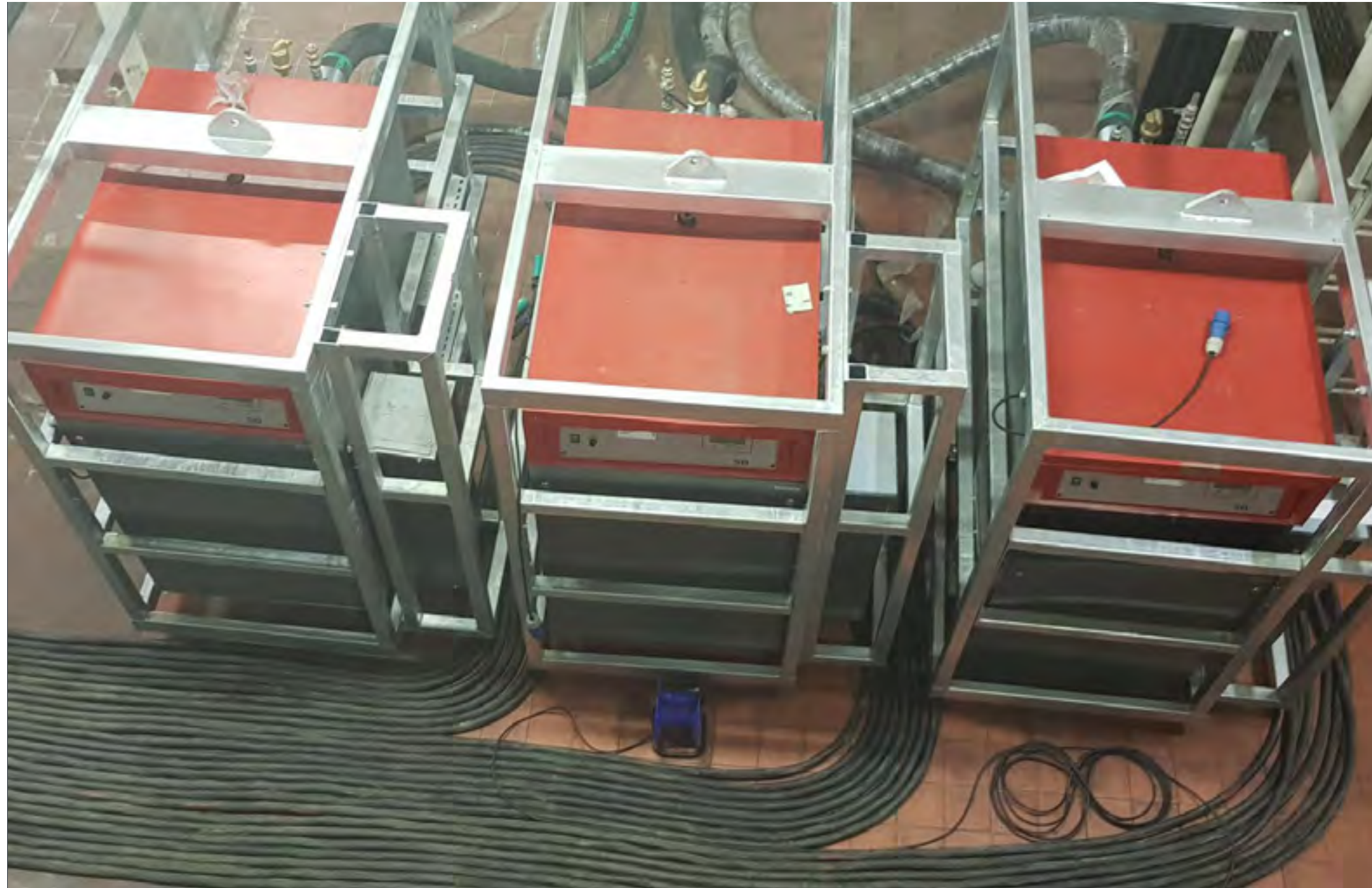
3 x 600 kW electric boilers for factory acceptance testing of data centre chillers.
