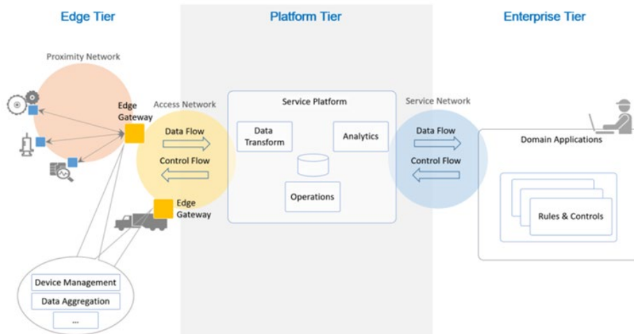
Figure 5: Three-tier IIoT system architecture.
