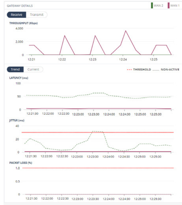
Figure 2: Monitor link health against target thresholds
